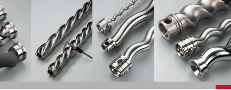
For our standard rotors we use stainless steel 1.4571 or AISI 316 Ti as well as tool steel 1.2436 vacuum-hardened to 61 HRC. Of course we also work with other materials if required.
